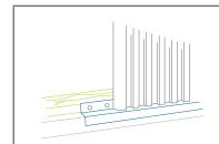
The side sheeting is sealed off at the bottom with base molding to guard against intrusion by rodents and insects.
